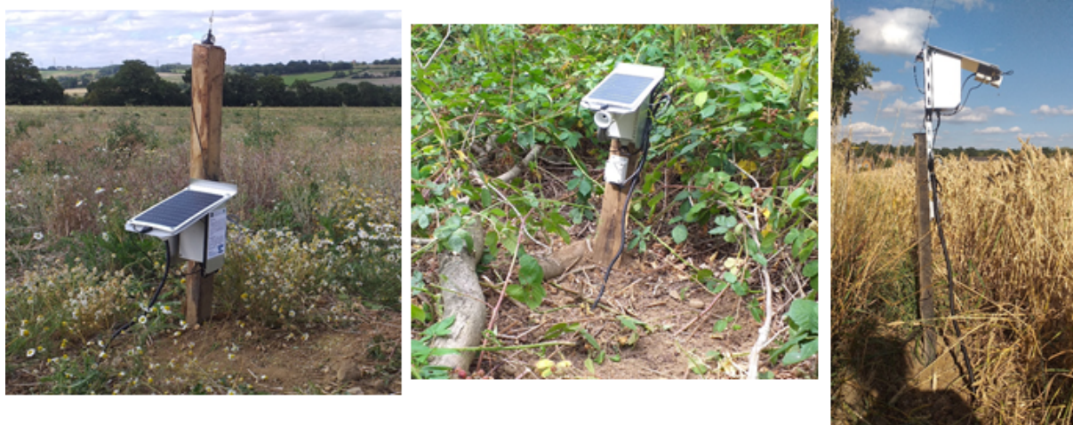
Figure 10: FreeStations equipped with soil moisture probes deployed as a transect across the Salmons Brook valley (Figure 8) in different current land use types. Left: set aside for woodland planting; middle: established woodland; right: arable farmland.
