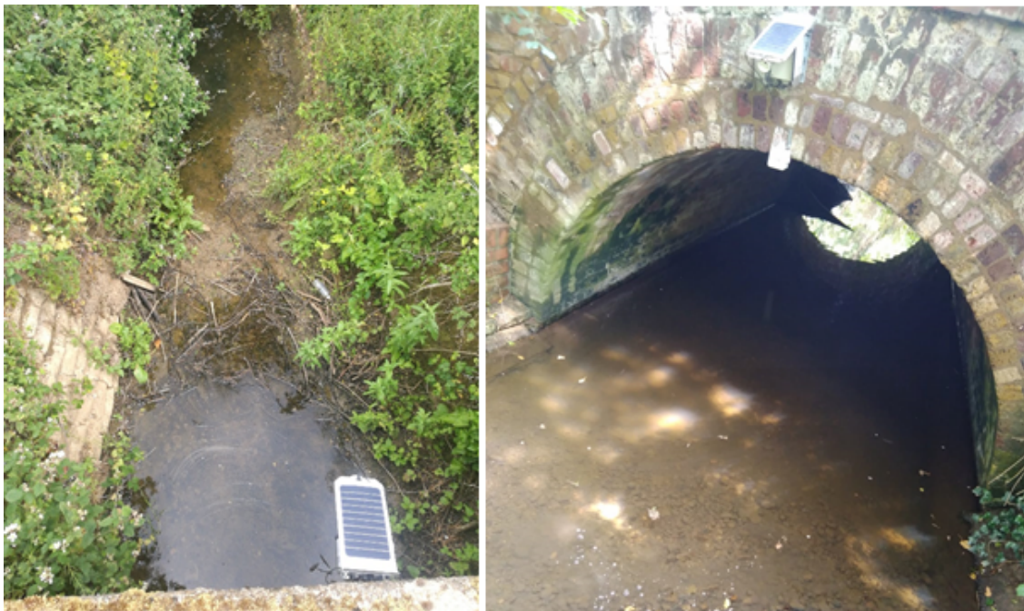
Figure 9: FreeStations equipped with water level sensors deployed on the Salmons Brook main watercourse. Left: mid catchment on a bridge on private farmland, right: at the bottom of the rural catchment catchment on a road bridge.
