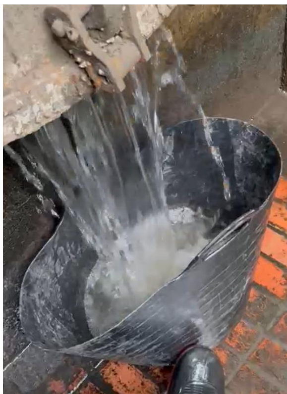
Figure 3: Still from a video of the flow measurement methodology using a bucket at the outfall.
